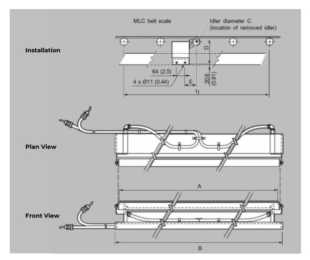
For pan supported belts, the belt should be cut out to allow the RLCS and at least two (preferably four) other idlers to be installed.
