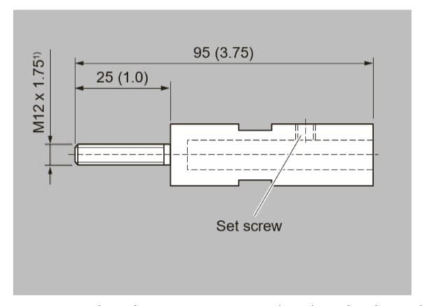
WS300 mounting using threaded shaft coupling, dimensions in mm (inch)
