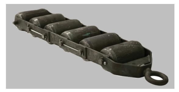
Rubbex Roller test chains are used for belt scale calibration when material tests are not practical. All test chains are bushed. Minimum length is 4 feet (1.2 m).
