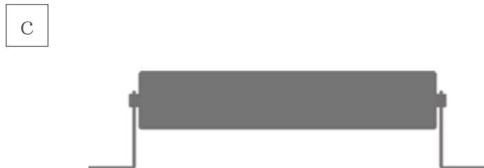
Flat carrier roller stand used to bulk handling material such as preparing Foundry sand, package and sort conveyor.
