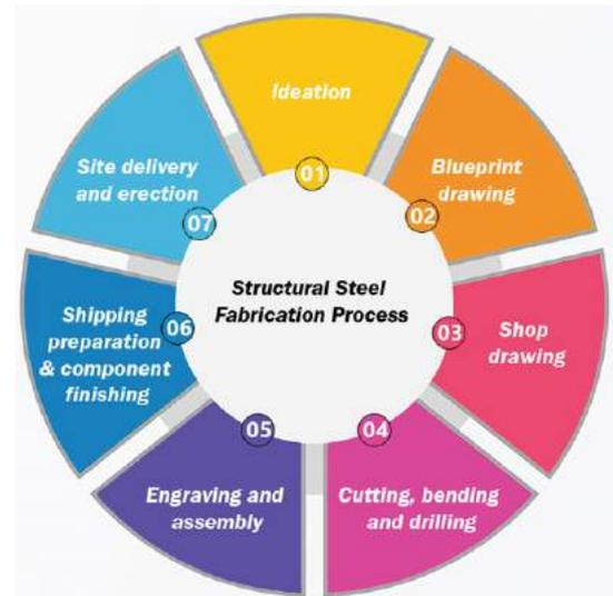
Structural steel fabrication is the process of bending, cutting, and modelling steel to form a structure. For structural steel fabrication pieces of steel are put together to make different structures that are usually of predefined sizes and shapes. It is a complex process that requires specialized knowledge, skills, and resources to complete successfully.
