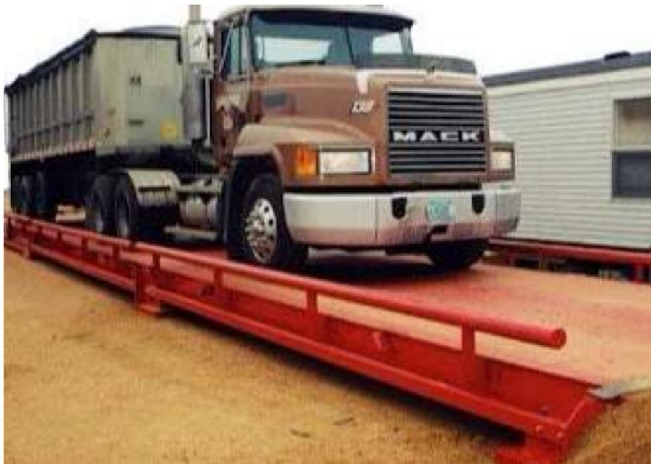
Weighbridges scales are mounted on a concrete surface and have an electronic or digital monitoring component that displays the weight of an entire vehicle.
