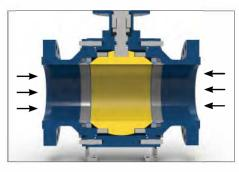
The Double Block and Bleed (DBB) feature is offered in both seat ring configurations (SPE and DPE). When the valve is in the closed position, the pressure is blocked in the body cavity by the pressure activated seat rings on both sides. Body cavity pressure can then be relieved by drain or vent.
