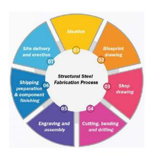
Structural steel fabrication is the process of bending, cutting, and modelling steel to form a structure. For structural steel fabrication pieces of steel are put together to make different structures that are usually of predefined sizes and shapes. It is a complex process that requires specialized knowledge, skills, and resources to complete successfully.
